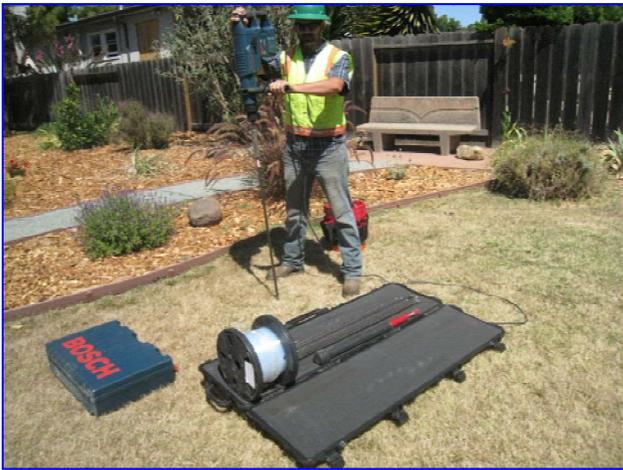
ERAS now has powered drilling and sampling equipment that enables us to collect soil gas (aka soil vapor) samples and shallow soil samples for laboratory analysis. The equipment includes drilling equipment and drilling rods that allow for driving of drill rods to depths of up to 10 feet for sampling depending on subsurface conditions.
